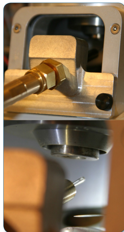
Figure 1: Photos of ASAP probe and glass capillary tip which supports the sample for analysis
