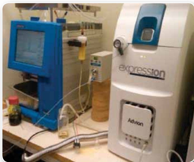
Online Flash/CMS UV Fractionation and Mass Confirmation
