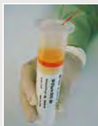
The sample gradually penetrates into the frit (filter) of a column.
