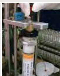
Connect the line of an instrument (lure adaptor) to a column.
