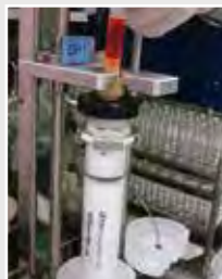
Insert the syringe containing the sample into the lure joint of a column.
